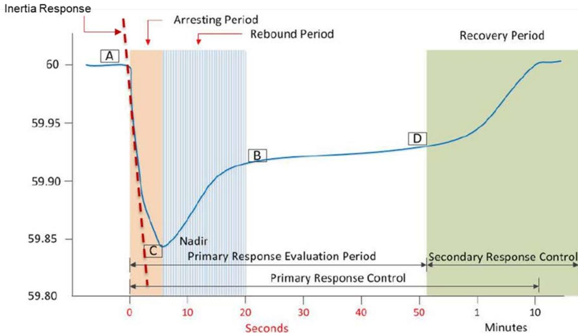
**Figure 3.1: Typical Frequency Excursion and Recovery**
