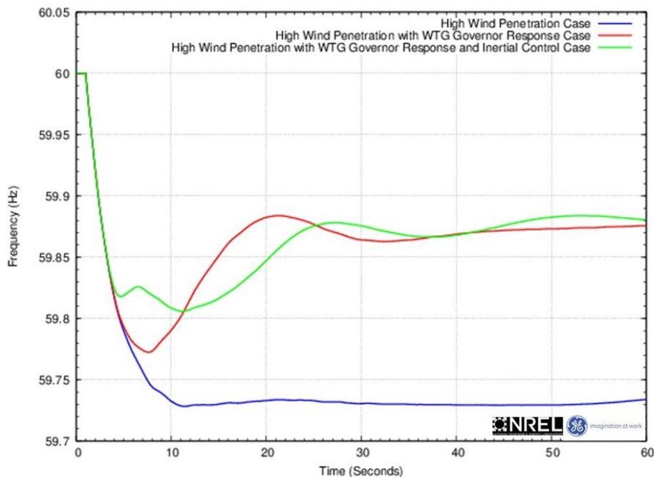
Figure 5.2: Illustration of Wind Turbine Frequency Controls<sup>69</sup>
